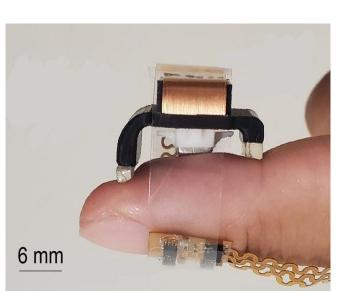
One device comprises a tiny magnet, wire coils, an accelerometer, a small rechargeable battery and Bluetooth capabilities.
